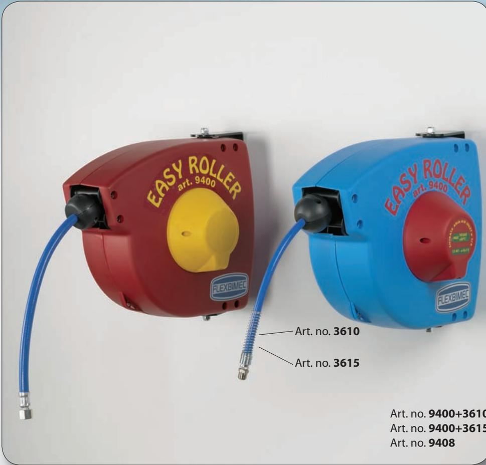
Automatic rewind, spring-driven hose reel, with plastic enclosure (made of nylon and polypropylene) and pivoting wall bracket, suitable for the use with compressed air and water (temperature range: -10°C – +60°C) and for hoses of 8 x 12 mm (or 10 x 14 mm) with a max. length of 15 m (or 10 m).
