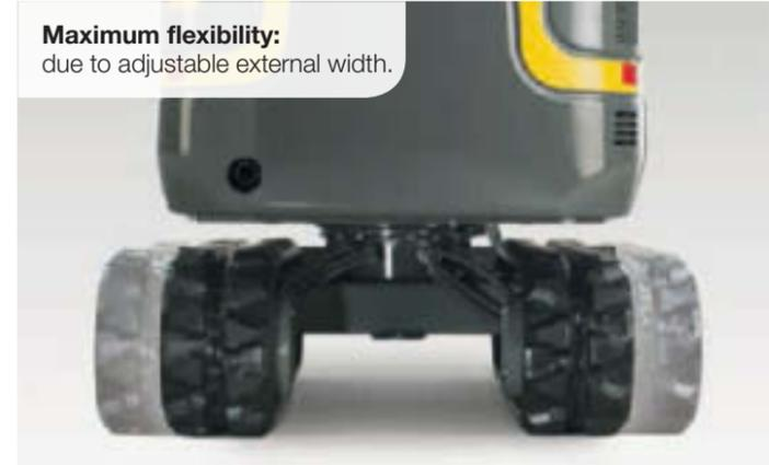
Telescoping travel gear is available for: 803, 803 dual power, 1404, EZ17, ET18, ET20
