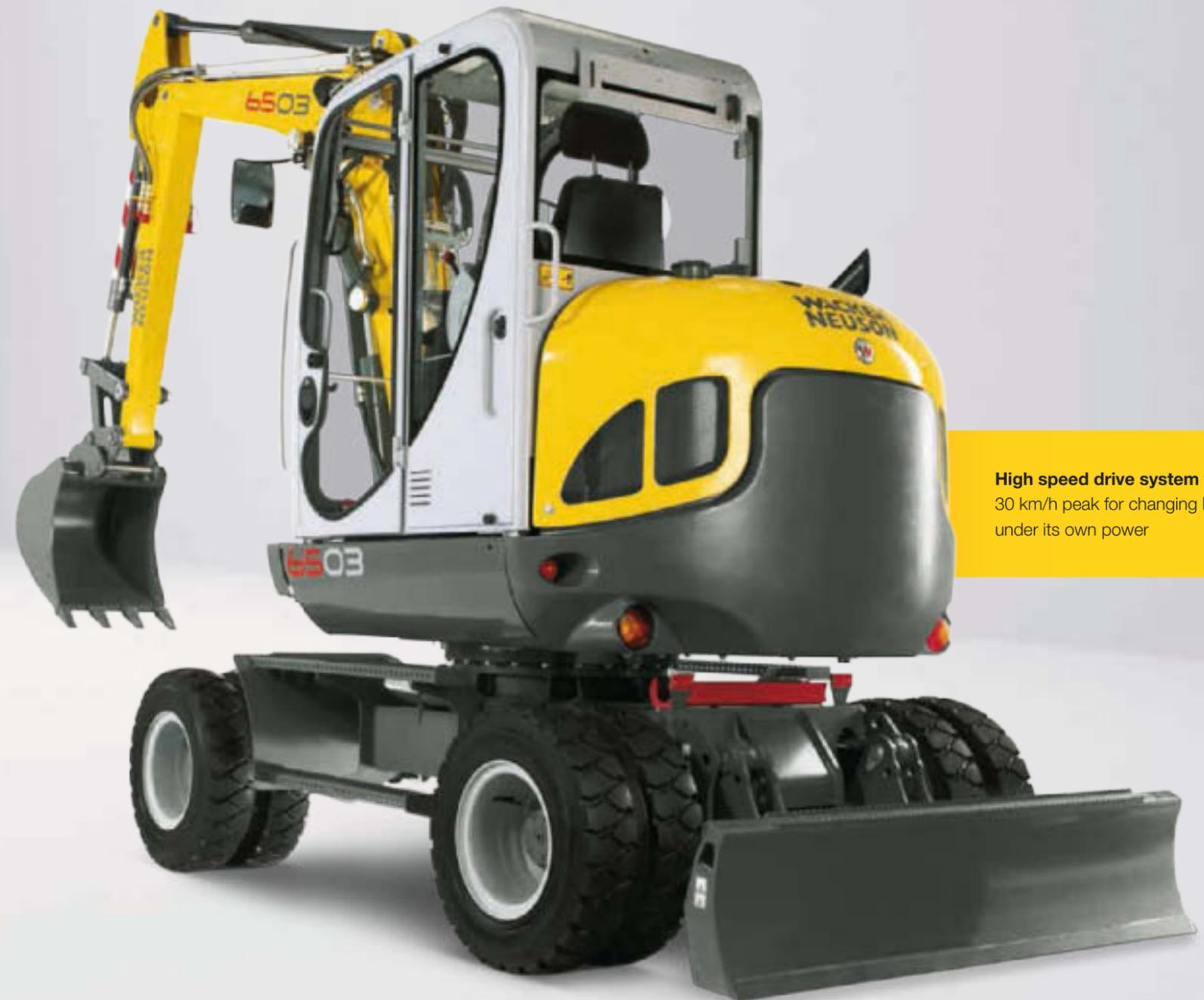
High speed drive system with up to 30 km/h peak for changing locations under its own power
