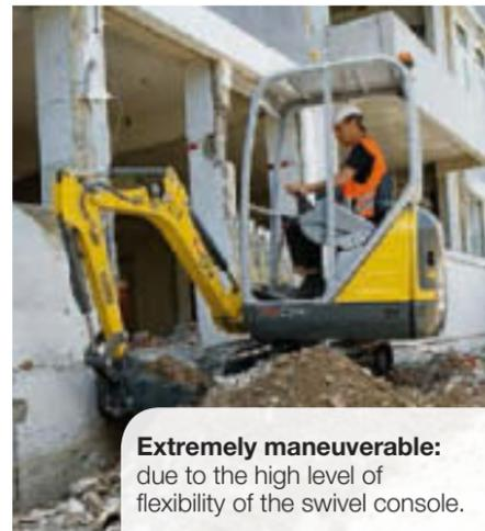
**Extremely maneuverable:** due to the high level of flexibility of the swivel console.
