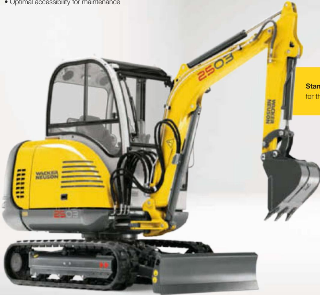
**Standard:** Auxiliary hydraulics for the dipper stick.
