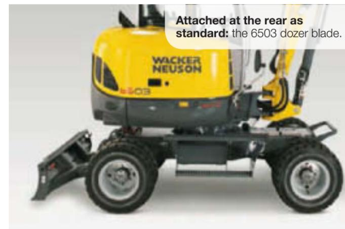
Attached at the rear as standard: the 6503 dozer blade.
