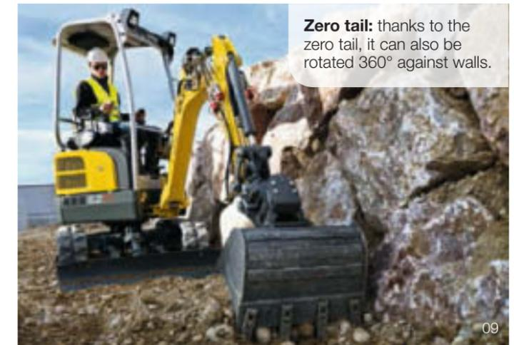
**Zero tail:** thanks to the zero tail, it can also be rotated 360° against walls.
