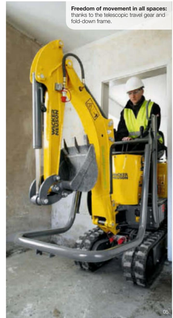
**Freedom of movement in all spaces:** thanks to the telescopic travel gear and fold-down frame.
