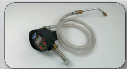
Art. no. 2824 Digital flow meter art. no. 2629 (see page 61!) with connection adapter for manual pumps, 1 m - outlet hose and rigid outlet with automatic anti-drip nozzle.
