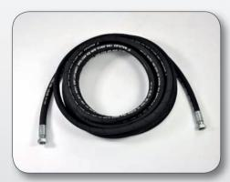
High pressure rubber hoses in accordance with SAE 100 R2AT, with swaged female BSP connection threads (swivel nuts), suitable for the supply of **grease** and **water** at high pressure. Internal structure in oil-resistant, synthetic rubber, coating in rubber highly resistant to abrasion, ozone and atmospheric influences. Reinforcement: 2 steel wire braided, highly resistant layers.
