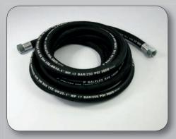
Low pressure rubber hoses in accordance with SAE 100 R6 – DIN EN 854, with swaged female BSP connection threads (swivel nuts), suitable for the supply of **diesel** and **water** at low pressure. Internal structure in oil-resistant, synthetic rubber, coating in rubber highly resistant to abrasion, ozone and atmospheric influences. Reinforcement: 1 textile braided and 1 steel wire braided layer.
