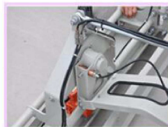
Screed plate can lock or loosen automatically
