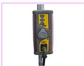
American Trimble laser receiver
